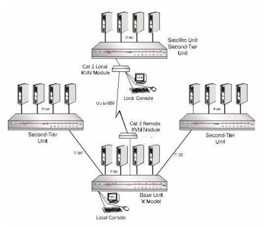
Figure 29 Two-Tier Configuration with Satellite Unit
